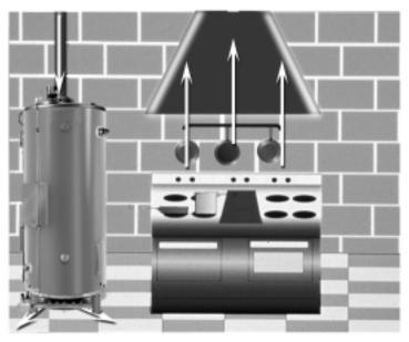
One common example is in a restaurant installation where exhaust vent equipment was not considered in sizing make-up requirements. This condition may result in air being backdrafted by the restaurant exhaust equipment through the heater causing the draft proving switch to open and/or erratic heater shutdown.
